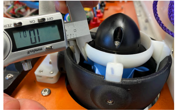
Figure 17: Shrouds meet IP2X standards
